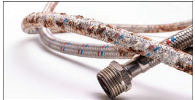
✗ Flexi hose in poor condition.
